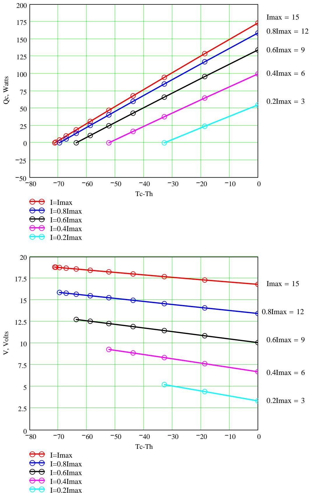
Qc -refrigerating capacity at cold side of the module (Watts),
